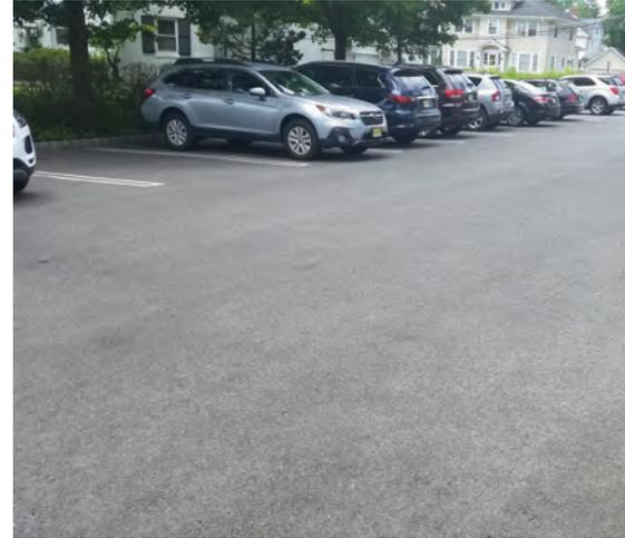
The turfgrass to the southeast of the building can be converted to a bioretention system to help capture, treat, and infiltrate stormwater runoff from the building's roof. Parking spaces in the western portion of the parking lot can be converted to pervious pavement to capture and infiltrate stormwater runoff from the lot. A preliminary soil assessment suggests that more soil testing would be required before determining the soil's suitability for green infrastructure.
